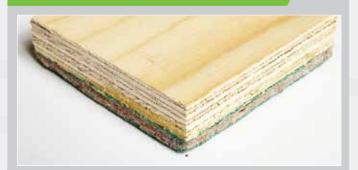
Hush-Ply 32 has been designed as an impact reducing floor panel that can be used as a structural or an overlay board. Offering an alternative to the standard chipboard finish, Hush-Ply 32 is especially suitable for areas requiring extra moisture protection, such as kitchens and bathrooms and offers an excellent surface for application of the final flooring finish, whether using ceramic tiles or wooden flooring.
