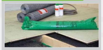
Hush Fill 6o Heavy Pugging is a granular mineral filler specifically designed to meet the required density of 8okgs/ m² at the 6omm regulation depth specified within UK Building Regulations for sound insulation between timber floor joists.
