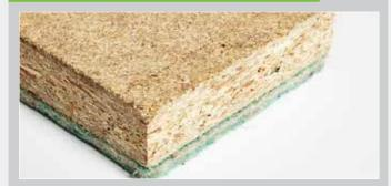
Hush-Panel 32 has been designed as an impact reducing floor panel, with added rigidity, that can be used as a structural or an overlay board. When used as a structural floor the stiffness of the upper layer accommodates wider joist centres, up to 600mm. A combination of the increase in mass and the Hushfelt™ resilient layer can produce superior results when used as part of a sound insulation system for separating floors.
