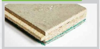
Hush Panel Cem 28 is a high mass acoustic floorboard that has been developed to increase both airborne and impact acoustic performance when used in an existing construction that is deemed to be very lightweight. By adding high amounts of mass to a lightweight construction the airborne noise performance is increased, something that doesn't normally occur when standard acoustic flooring is used.
