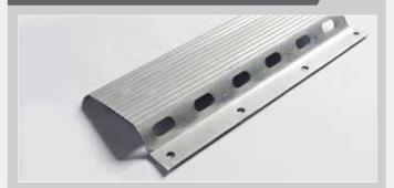
Hush Bar resilient bars are used to optimise acoustic performance by virtually decoupling a lining from a ceiling or wall structure. By using the Hush-Bars the airborne and impact sound transmission is significantly reduced. The Hush-Bars are one of the most important elements of a system to ensure compliance with the Building Regulations for sound transmission through separating ceilings and walls.
