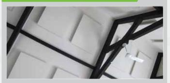
The Hush Absorber 50A is a Class A Absorber which consists of fabric wrapped 50mm thick acoustic foam, with built in support frames to allow for bracket fixing to provide an air void behind the absorber for enhanced acoustic performance.
