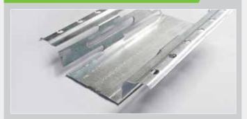
Hush bars are used to optimise acoustic performance by virtually decoupling a ceiling or wall lining from it's structure. This significantly reduces sound transmission through the floor, ceiling and wall structures. The Hush-Bar Deep resilient bar creates a larger void within a construction and allows high mass boards to be used. The Hush-Bar Deep can provide enhanced acoustic performance compared to standard resilient bars when used with a recommended lining.
