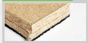
Hush Panel 33 has been designed as a versatile but high performing acoustic flooring to be used in conjunction with a timber joisted structure. The unique combination of Eco-Friendly acoustic felt and a rubber barrier mat make the product perform to all UK Building Regulations Requirements whether this be Approved Document E (England & Wales), Section 5 (Scotland) or Part G (Norther Ireland).
