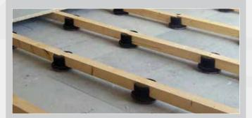
Hush Cradles have been designed as a timber batten support with an infinitely adjustable thread, allowing for precise levelling across uneven sub-floors without the use of fiddly packers.
