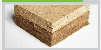
Hush Panel 48 has been designed to enable an increase in floor height within refurbishment, change of use and new build projects. The combination of the Hush Slab 30<sup>™</sup> resilient layer to the underside and high density upper layer offers excellent acoustic qualities. The resilient layer can also take care of minor undulations of the floor surface.
