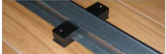
The Hush Bar Enhanced damping clips ensure total isolation but also as they are fixed from both sides they ensure a much greater load bearing capacity than most standard systems – up to 80 kgs per m<sup>2</sup>. (please check with Hush Acoustics Technical Team regarding loading information).
